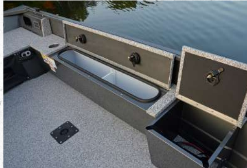
Outfitter 160 port side livewell and battery box
